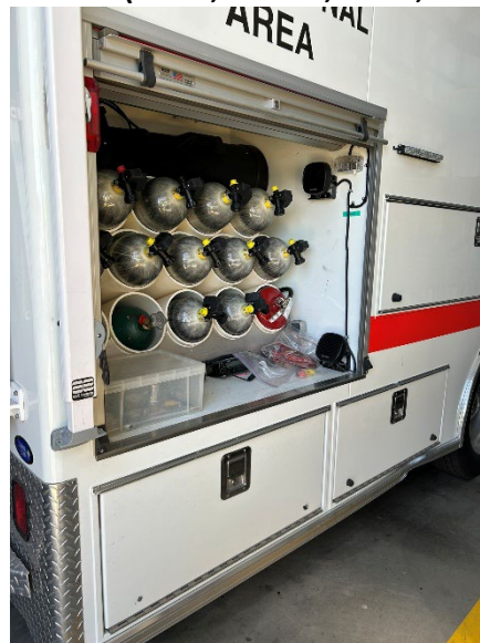
SCBA Tank Storage- 1 hr. tank = 20 lbs. moved from ground up to 64 inches
